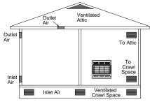
Figure 3 - Ventilation Air from Outdoors
